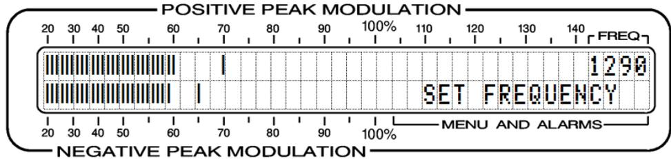
The SEL buttons may be used to set the receive frequency, which is always displayed in the upper-right corner of the LCD screen under **FREQ**. The SEL buttons may be incremented in single 1kHz steps, or held-down to scan quickly up and down the band.
