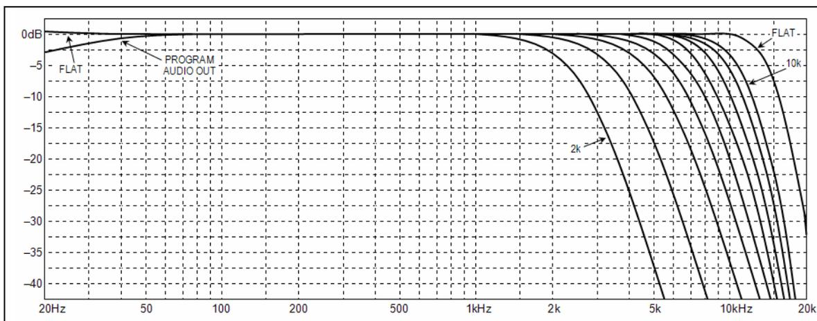
**Figure 1** - Model 525 Off-Air Measurement Response (FLAT) and Program-Audio Cutoff Options
