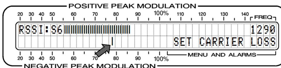
The single LCD segment below the RSSI display corresponds to the alarm trip point. This segment is identified here with an arrow. It may be positioned with the SEL buttons anywhere in the RSSI metering range. The carrier loss alarm is activated immediately whenever the RF level falls below the set point.
