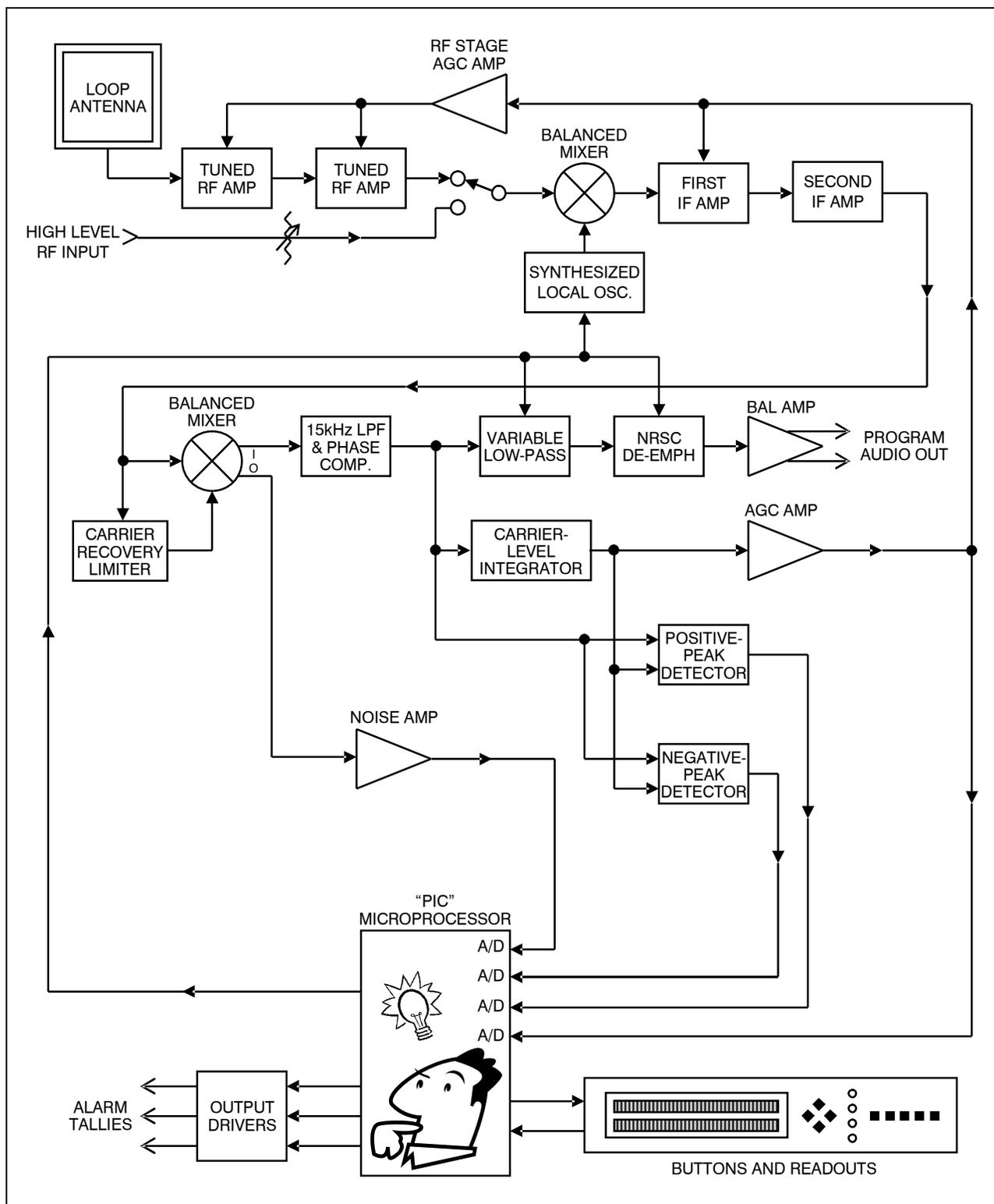
Figure 4 - Block Diagram, Inovonics Model 525
