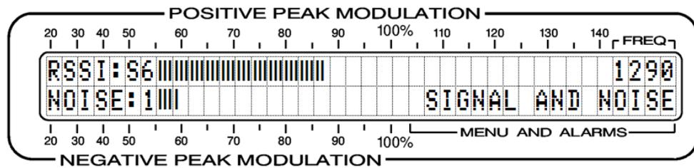
The upper bargraph now represents a Received Signal Strength Indication, or RSSI. The quasi-log LCD bargraph gives a relative indication of incoming RF level, and a numerical 'S' value is displayed to the left of the bar. This will vary between S0 (zero) and S9. An increase of one S unit represents a signal increase of 6dB. Generally a reading of S8 or higher is required to assure modulation measurement accuracy.
