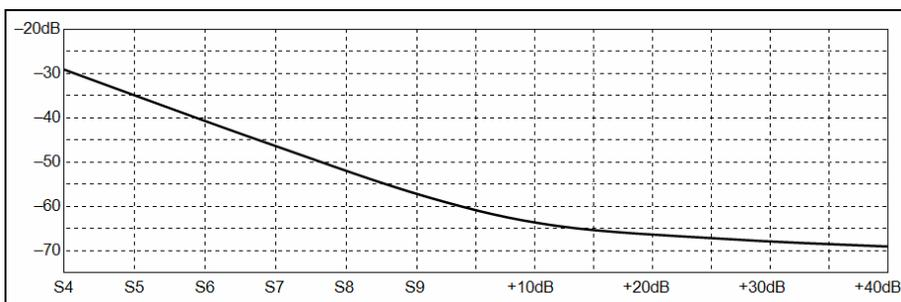
**Figure 3** - Output Noise vs. RSSI
