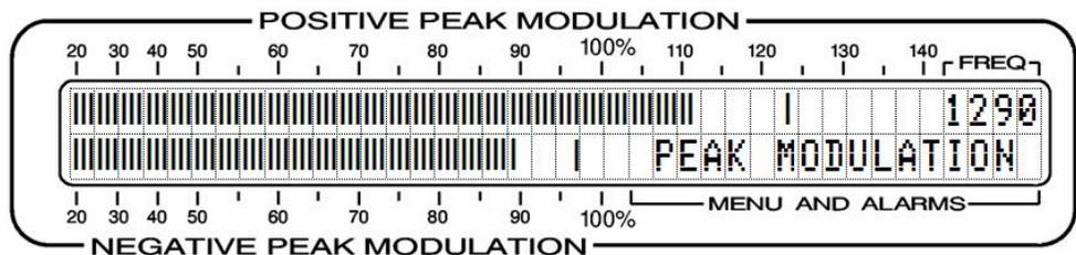
The two bargraphs show positive and negative carrier modulation independently and concurrently. The bargraphs will follow the modulation to the extent that an LCD can keep up with rock 'n' roll, and single segments representing the highest positive and negative peaks will 'hang' above the bars for about a second to ensure that the highest instantaneous value will be displayed with no ambiguity.
