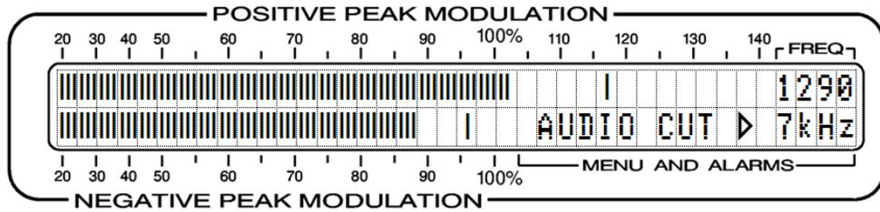
The SEL buttons set the audio cutoff to FLAT, or in 1kHz increments from 10kHz down to 2kHz. Figure 1 on Page 5 shows a plot of this family of curves. The frequency indicated by the display is the -3dB point of a fourth-order (24dB/octave) low-pass filter. This cutoff applies only to the rear-panel PROGRAM AUDIO OUT connector and to the front-panel PHONES jack.
