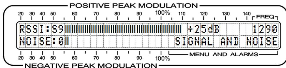
AGC action of the 525 can handle inputs up to 40dB over S9. When the AGC reaches the end of its control range, the word OVERLOAD! appears to the right of the bar as shown on the next page.
