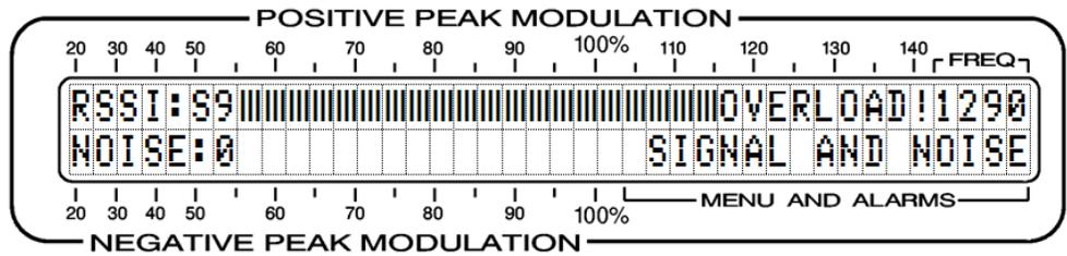
Modulation measurements cannot be trusted as accurate either at very low signal levels or with an input overload. When OVERLOAD! appears in normal operation, either reduce the antenna signal by replacing the loop antenna with a short length of wire, or use a direct, high-level input connection and adjust the rear-panel LEVEL SET pot for an indication between S9 and S9+40dB.
