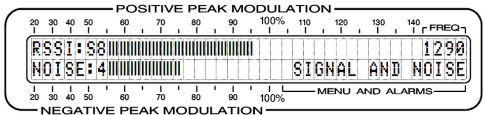
This noise measurement utility displays a relative level of “stuff that shouldn’t be there,” which may include modulation splatter or spillover from adjacent stations. With 1kHz tuning increments, it is easy to be off-frequency, which is another condition that will cause a high noise reading.
