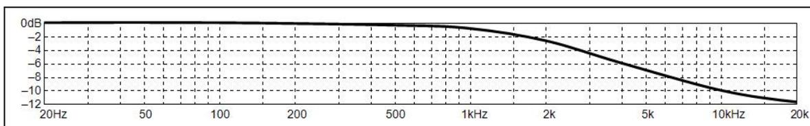
**Figure 2** - NRSC De-Emphasis Curve for AM Broadcasting
