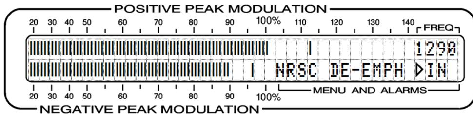
De-emphasis is normally left IN for listening, but may be switched OUT when making measurements through the rear-panel PROGRAM AUDIO OUT connector. Again, de-emphasis is automatically switched out when AUDIO CUT is set to FLAT. As with the audio bandwidth selection, de-emphasis affects only the audio outputs and has no effect on modulation measurements.
