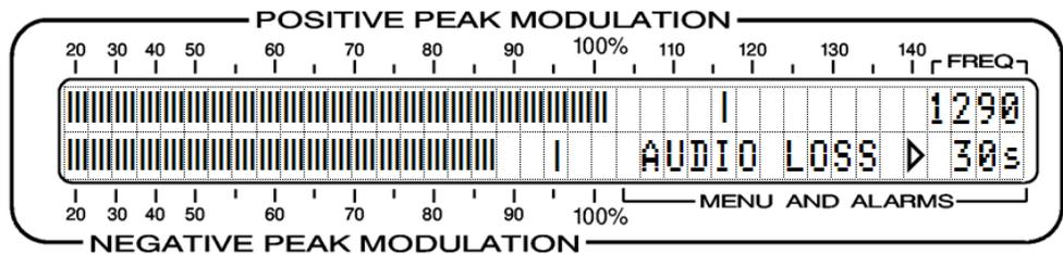
SEL buttons are used to set the alarm timeout to any period between 5 seconds and 120 seconds (2 minutes).
